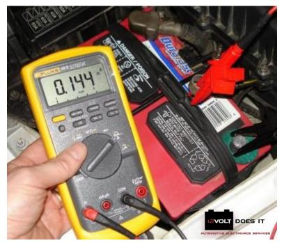
Measuring current draw with a multimeter. This can help you find components and circuits that are drawing too much current from the battery and charging system. Current draw on most vehicles should be less than 40 to 50 milliamps after 30 minutes once the engine is turned off.
